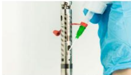
Figure 1.18 Lubricate the tube seal through either of the tube seal flush ports
