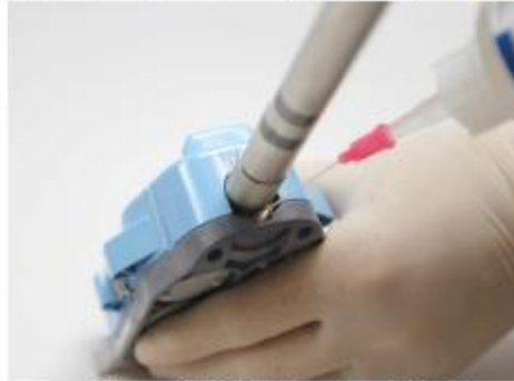
Figure 1.19 Lubricate the roll joint
