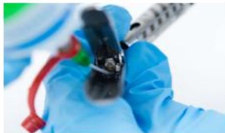
Figure 1.14 Lubricate the proximal crotch of jaws
