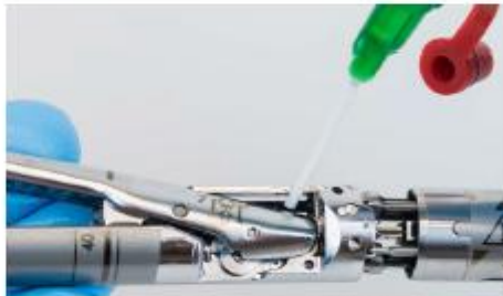
Figure 1.15 Lubricate the lead screw
