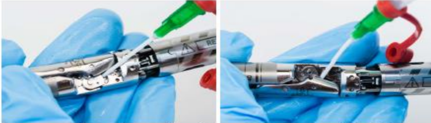
Figure 1.16 Lubricate the grip cable pulleys (two pulleys, one on each side of the jaws)
