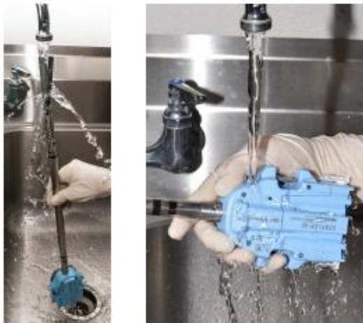
Figure 1.13 Rinse outside of entire instrument
