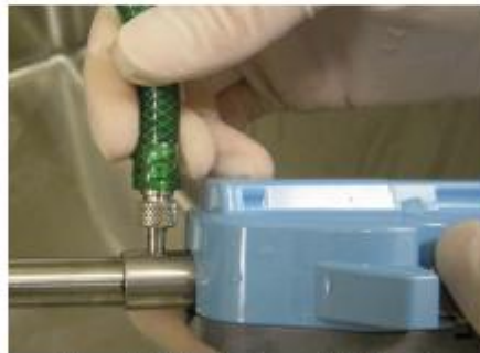
Figure 1.7 Flush primary flush port
